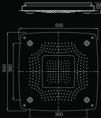
**OSA-CHR-70021:** Rainjoy+ Shower 500X500mm AISI 304 stainless steel in polished finish with RGB LED lights remote control & with installation kit for false ceiling
